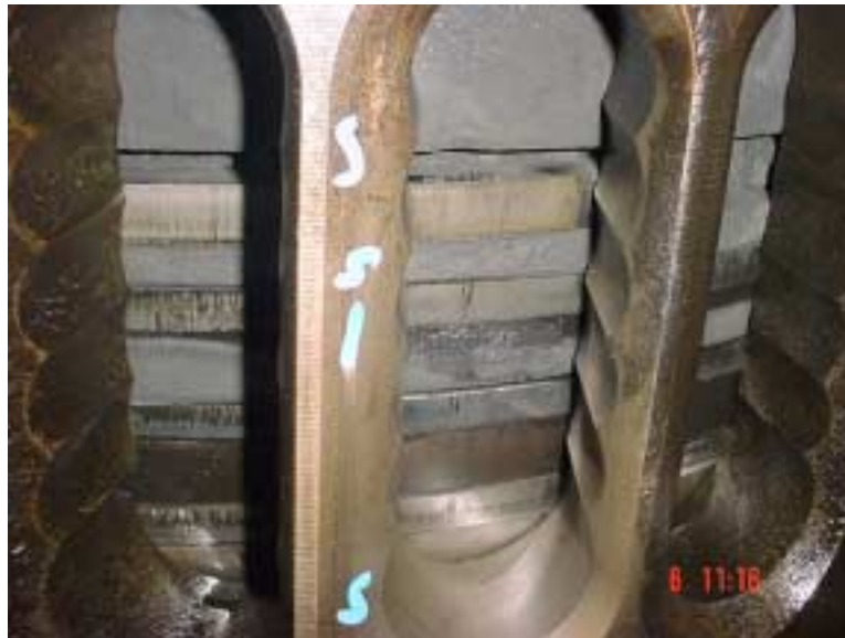
Picture 2 – Condition Unit 1 Fig 16 traced to excessive ring groove clearance and broken 1 st ring.
