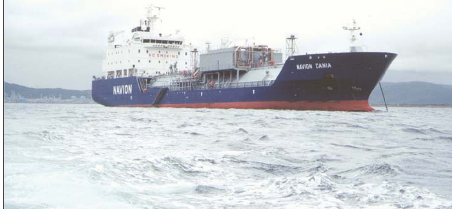
Fig. 29: M/V Navion Dania with SCR catalytic reactor installed
