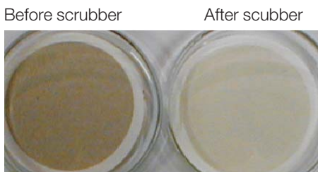
Fig. 21: PM on filters before and after scrubber
