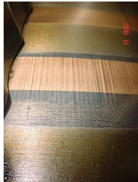
Initial wearing in of copper band on the piston skirt of Unit 4. Pic 4 – Ship A (Inspection on 17 th March 03)
