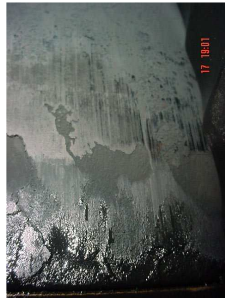
Deposits on Unit 4 piston top land abrading the liner wall. Pic 3 – Ship A (Inspection on 17 th March 03)
